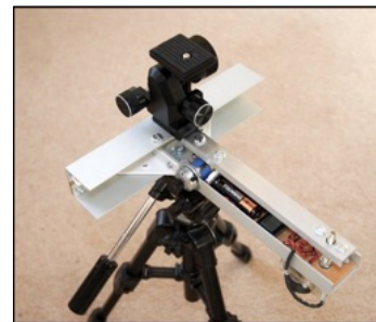
DIY star tracker 'K2' designed and built by Steve Used 2007–2013
