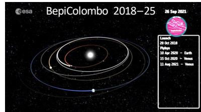
A flyby can accelerate **or** decelerate, but in both cases fuel is saved.
