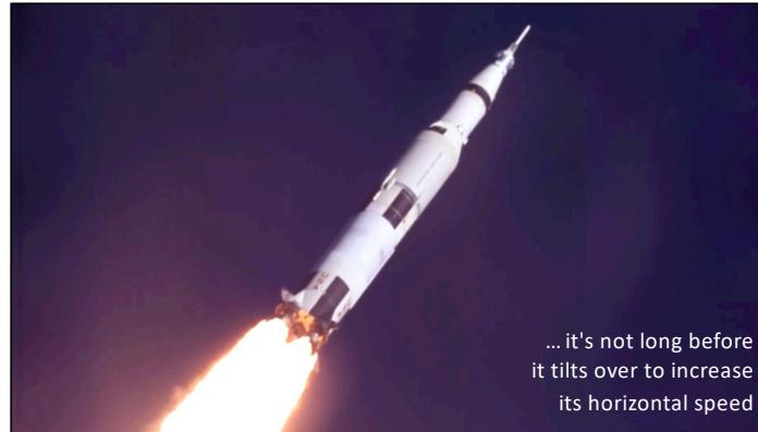
A photograph of a Saturn V rocket launching vertically from a launch pad. The rocket is oriented vertically, with its engines at the base. A large plume of white smoke and fire is visible at the base. The text '... it's not long before it tilts over to increase its horizontal speed' is overlaid on the right side of the image.
