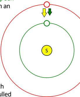
There is a red orbit at just the right distance such that the extra pull from the Earth makes the red object orbit faster with a period of 1 year.
