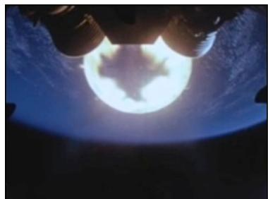
Engine exhaust plumes are not visible in a vacuum
