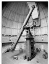
Telescopes have come a long way in the 400 years since Galileo. Refractors (using lenses) gave way to reflectors (using mirrors) over a century ago as lenses larger than ~1 m in diameter are impractical.
