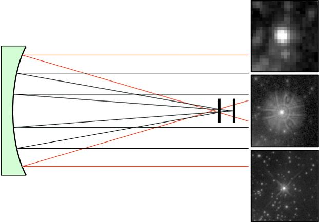
The diagram illustrates spherical aberration. On the left, a green concave spherical mirror reflects parallel light rays. The central rays (black) focus at a point further from the mirror than the peripheral rays (red). This causes the light to form a blurred spot instead of a sharp point. To the right, three panels show the resulting star images: a blurred central spot, a star with a diffuse halo, and a star with a large, irregularly shaped halo.
