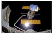
For the HST, the resolution is more than 10 times better. The 2.4 m diameter mirror in the HST was a result of the restriction that the entire telescope had to fit inside the cargo bay of the space shuttle.
