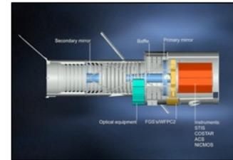
The cameras are labelled 'wide-angle' or 'high-resolution' depending on the effective focal length at which they are used (HST nominal FL ~58 m).
