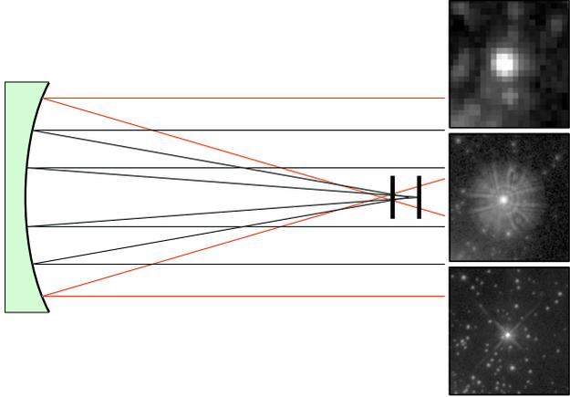
The diagram illustrates spherical aberration. On the left, a green concave spherical mirror reflects parallel light rays. The central rays focus at a point further to the right, while the outer rays focus at a point closer to the mirror. This results in a blurred image on the right, shown in three panels: a single star, a star cluster, and a field of stars, all appearing out of focus.
