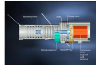
The cameras are labelled 'wide-angle' or 'high-resolution' depending on the effective focal length at which they are used (HST nominal FL ~58 m).
