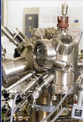
The STM is sealed inside an ultra-high vacuum vessel ( $10^{-13}$  atms) to keep it and the sample surface clean.
