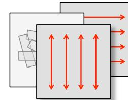
Place a sheet of plastic between them and see what happens. If the plastic has strips of sticky tape on it, they appear coloured dependent on the thicknesses of the tape.
