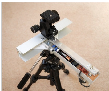
DIY star tracker 'K2' that I designed and built Used 2007–2013
