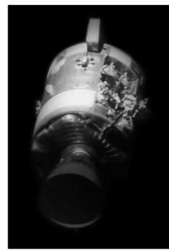
A fan inside one of the oxygen tanks had faulty wiring insulation, so when the tank was stirred a spark caused the oxygen tank to explode, damaging the fuel cells and blowing out a side panel of the SM.
