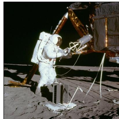
Alan Bean (Apollo 12) removes the plutonium fuel cask from the LM to transfer it to the RTG in front of him that powers the experiments on the lunar surface.
