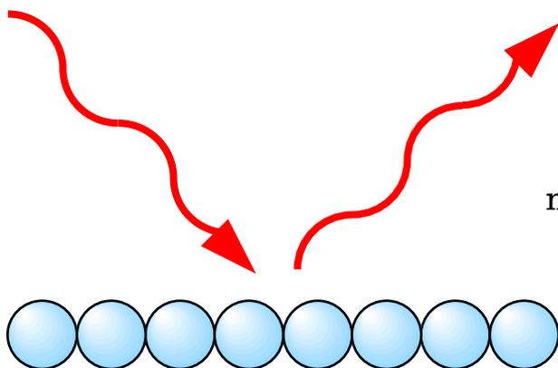
Shine light onto a surface and see how much gets reflected, scanning through a range of wavelengths (or frequencies). When the frequency matches the resonant frequency of a molecule sitting on the surface, some light will be absorbed – some of the photons will be absorbed by the molecule, increasing the amplitude of its vibration.
