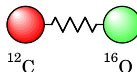
However, if one of the atoms is bonded to the atoms in a surface, then its movement will be greatly restricted. If the molecule sits on a surface with the O atom bonded to the surface, then the C atom will be free to oscillate up and down and so will undergo simple harmonic motion. Similarly for the case if the C atom is bonded to the surface, but because the masses of the O and C atoms are different, the resonant frequency of vibration will be different for these two geometries.
