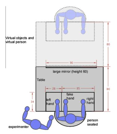
**Fig. 1.** A diagram of the apparatus in the mirror condition in Experiment 1. All measures are in cm. The upper grey objects are virtual objects visible in the mirror. The rectangle around the hands is the occluder. The same table was used in the direct view condition with the top part of the occluder removed and the mirror covered.
