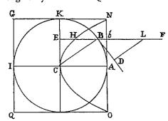
strike it perpendicularly in b, as LD is to LB, or BE to BC. Again; the efficacy of this force to move the globe, according to the direction of its incidence FB or AC, is to the efficacy of the same to move the globe, according to the direction of its determination, that is, in the direction of the right line BC in which it impels
