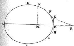
GH shall be perpendicular to the axis in the point of contact B, and FG, HI may be inclined to GH in the angles FGB, BHI of 135 degrees: the solid arising from the convolution of the figure ADFGHIE about the same axis AB will be less resisted than
