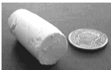
Photograph (left) and electron micrograph (right) of an emulsion templated material prepared using supercritical CO 2 [8]
