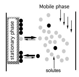
The different forms of liquid chromatography differ in the nature of the stationary and mobile phases. In the most common forms of chromatography, the stationary phase consists of an insoluble material (usually in beaded or granular form, e.g. cellulose or polystyrene) that is packed into a column and through which the mobile phase (containing the solutes) can flow.
