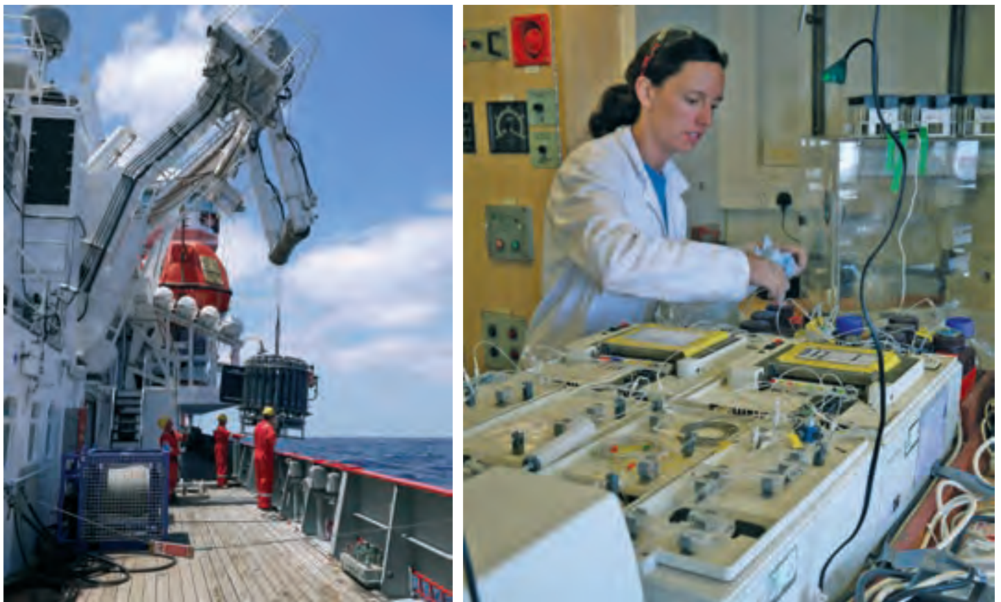
Figure 4 Left: an instrument package being deployed into the ocean to collect information. The package is lowered down to the seabed, sending back data including temperature, salt concentration and the amount of chlorophyll in the water. The grey bottles can be snapped shut at different depths, trapping seawater that is then analysed for phytoplankton and nutrient concentrations back aboard the research vessel (right)
