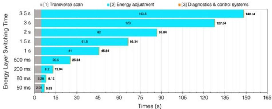
*Impact of energy layer switching time on beam delivery time for an example head & neck case.*
