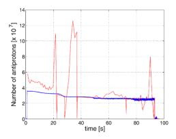
Measurement of the number of antiprotons during an AD cycle. In blue is shown the measurement from the new CCC device, and in red is the measurement from the existing monitor based on the analysis of the beam Schottky noise.
