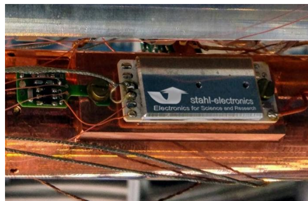
The CX4 amplifier (Stahl-Electronics) connected to the detection electrode.
