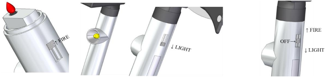
Figure 13. Integrated figure of a lighter button and flashlight switch.
