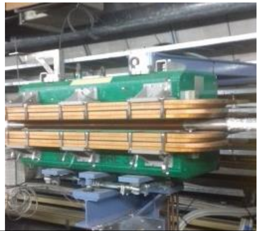
Here is a dipole magnet (A magnet with 2 poles) from the HERA tunnel
