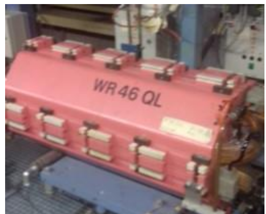
Here is a Quadrupole magnet (A magnet with four poles) from the HERA tunnel
