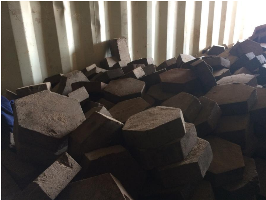
Some of the cement blocks made from melted down plastic and sand
