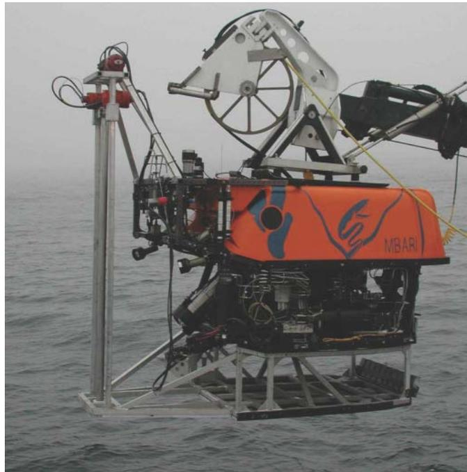
**Monterey Bay Aquarium Research Institute's remotely operated vehicle 'Ventana' with attached vibracoring system for sampling seafloor sediments. (Photo: E. Sumner)**
