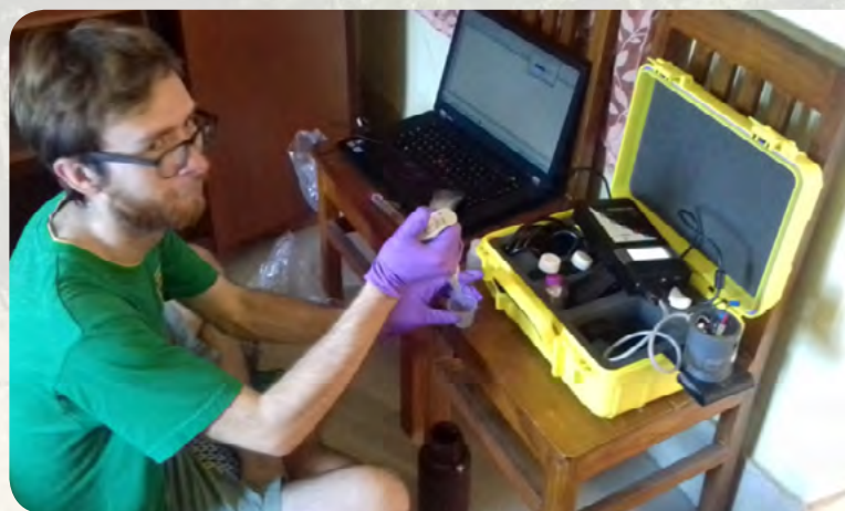
On-site analysis of arsenic in West Bengal, India, September 2018. Jay Bullen (Imperial College London), performing arsenic detection by voltammetric techniques.
