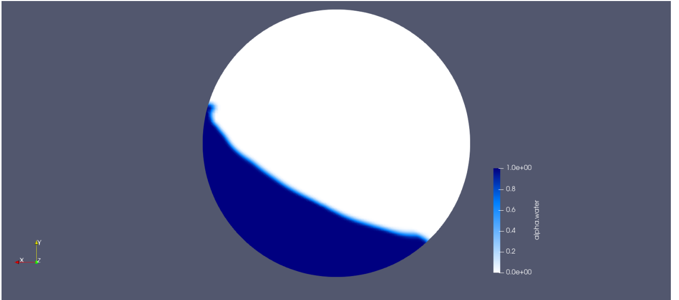
Figure 1. Snapshot of isothermal water sloshing simulation performed using OpenFOAM's Volume of Fluid (VOF) solver interFoam , which employs the MULES (Multidimensional Universal Limiter for Explicit Solution) algorithm for interface compression. The volume fraction scalar field \alpha is shown, where dark blue indicates the water region ( \alpha = 1 ) and white represents the air region ( \alpha = 0 ), and light blue indicates diffused interface between phases.
