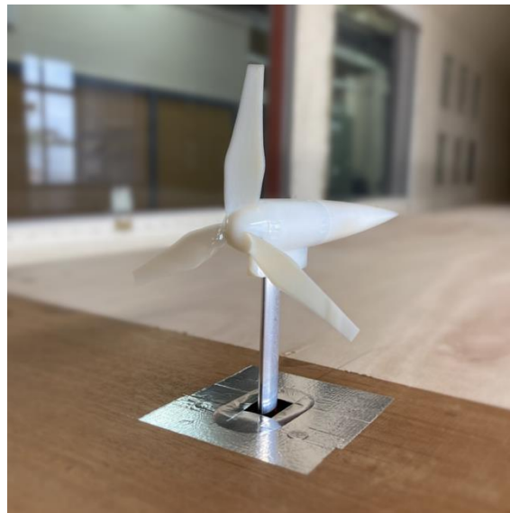
Figure 1. Miniature wind turbine. This turbine employs strain gauges at the base of the turbine tower below the ground board (not pictured) to measure the torque and drag it experiences. The turbine rotor used here is WIRE-01, by Bastankhah and Porté-Agel [2] and modified by Sampath [3].
