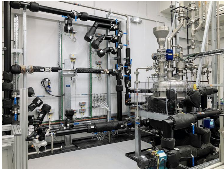
Figure 1. Image of the hydrotransport pipe loop, as part of the MULTIForm facility.
