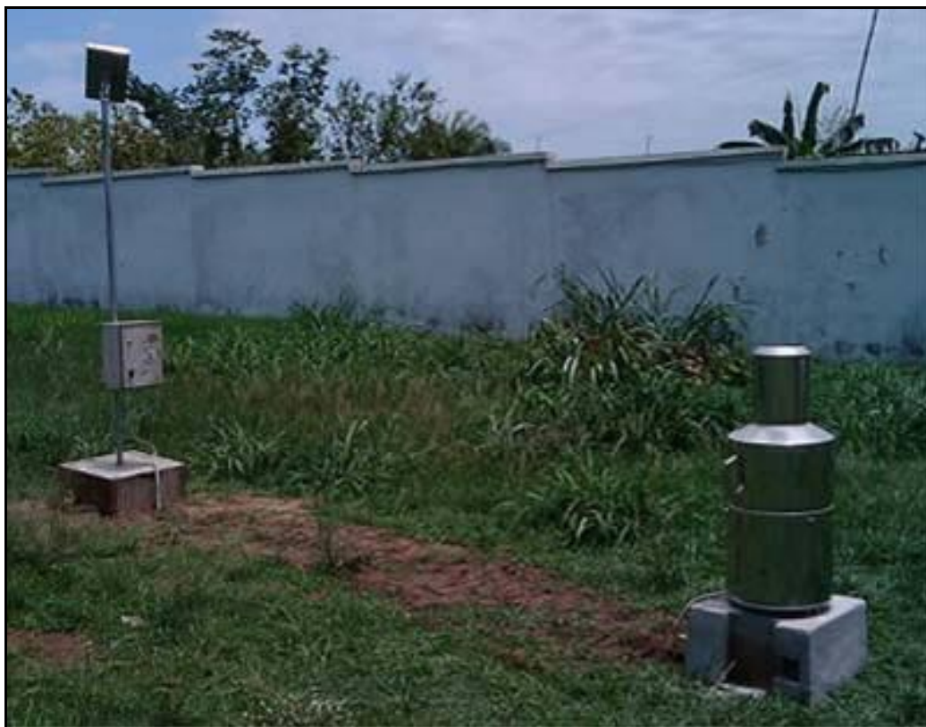
Figure 6: Pluviometer and solar power supply on the ground of the Emena hospital in Kumasi (Ghana) in April/May 2010.
