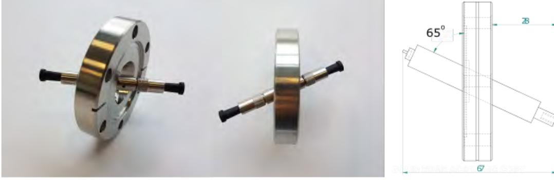
FIGURE 5.4: Pictures of the optical feedthrough, which was designed to use for gas jet velocity measurements. The optical feedthrough is going to be coupled with the light from the laser, and as a result the light axis has a fixed angle between the laser and the gaseous target.
