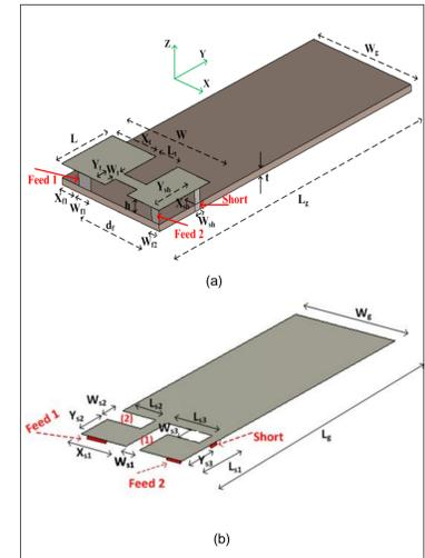
Fig. 2 Geometry of the proposed antenna
