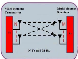
Fig. 1 MIMO system configuration
