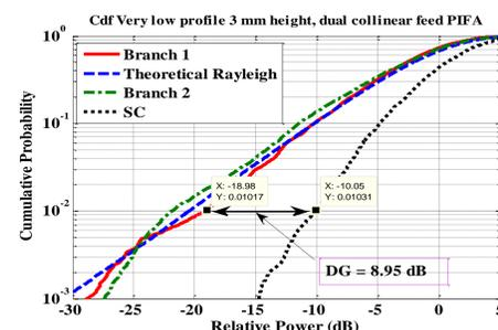
Fig. 8 Measured apparent diversity gain
