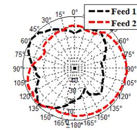
Fig. 6 Measured radiation pattern in YOZ plane @ 2.4 GHz
