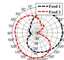
Fig. 5 Measured radiation pattern in XOZ plane @ 2.4 GHz
