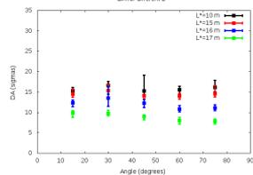
Figure 5. Dynamic Aperture comparison between optical designs with different  $L^*$
