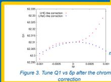
Figure 3. Tune Q1 vs  $\delta p$  after the chromatic correction
