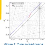
Figure 2. Tune spread over a momentum spread  $\delta p = \pm 0.001$  over a resonance map up to order 10.
