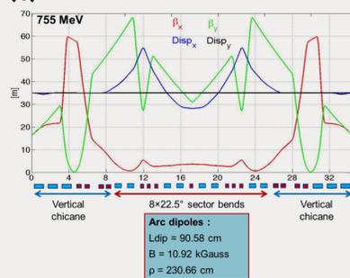
It includes a two-step achromat spreader and a mirror symmetric recombiner to direct the beam into the appropriate arc. The vertical dispersion introduced by the first step bend is suppressed by the quadrupoles located appropriately between the two stages.
