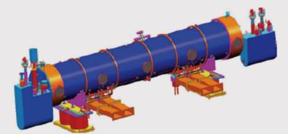
The cryo-cavity module being designed by the CERN-Jlab-Mainz collaboration. Image credit: SRF Institute, Jefferson Lab.
