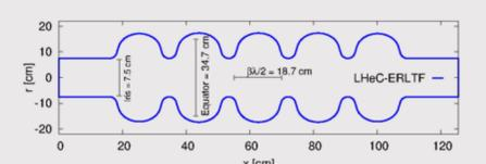
Approximate dimensions of a 5-cell cavity for ~802 MHz
