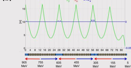
Figure 5. Concise representation of multi-pass ERL linac optics for all six passes, with constraints imposed on Twiss functions by 'sharing' the same return arcs by the accelerating and decelerating passes. Green and blue curves show, respectively, the evolution of the beta-functions amplitude and the horizontal dispersion for Linac 1 (a) and Linac 2 (b).
