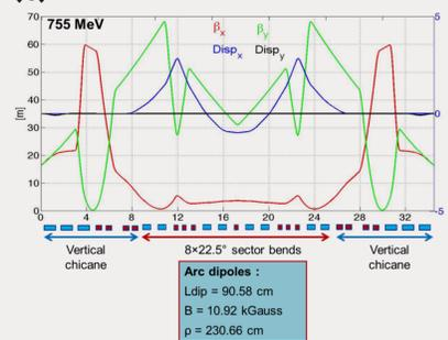
It includes a two-step achromat spreader and a mirror symmetric recombiner to direct the beam into the appropriate arc. The vertical dispersion introduced by the first step bend is suppressed by the quadrupoles located appropriately between the two stages.
