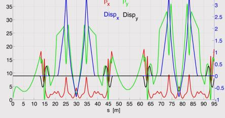
Complete lattice for Pass 1 including Linac1 (5 MeV to 155 MeV), Arc1 (155 MeV), Linac2 (155 MeV to 300 MeV), Arc2 (300 MeV).
