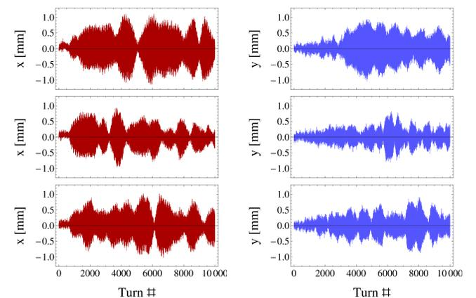
Measured trajectories while driving with AC dipole in both planes, for three beam pulses.
