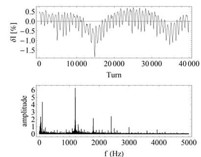
Variation in measured focusing quadrupole magnet current (top) and frequency spectrum of current (bottom).
