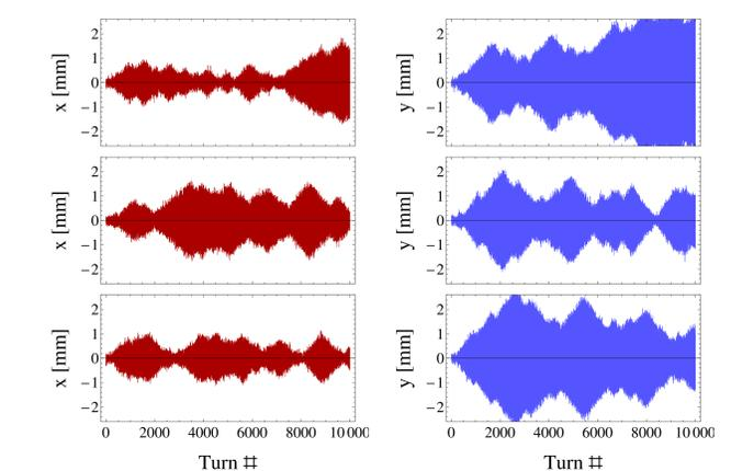
Simple tracking simulation including measured quad ripple, showing small and irregular beam response.
