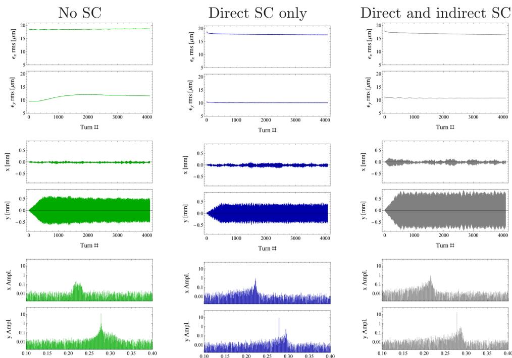
RMS emittance evolution, beam trajectories, and beam trajectory spectra from PTC-Orbit simulations with AC dipole excitation in vertical plane only. Three cases are shown: without SC effects, with direct SC only, and with both direct and indirect SC.
