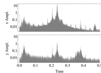
Spectra from tracking simulation with quadrupole noise at 296 kHz and 32.5 kHz.
