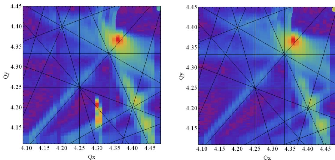
Tune scans performed with  $Q_x$  fixed,  $Q_y$  varied from 4.45 to 4.10. Closed orbit distortion is not corrected. Losses occur along  $Q_x \approx 4.30$  line.
