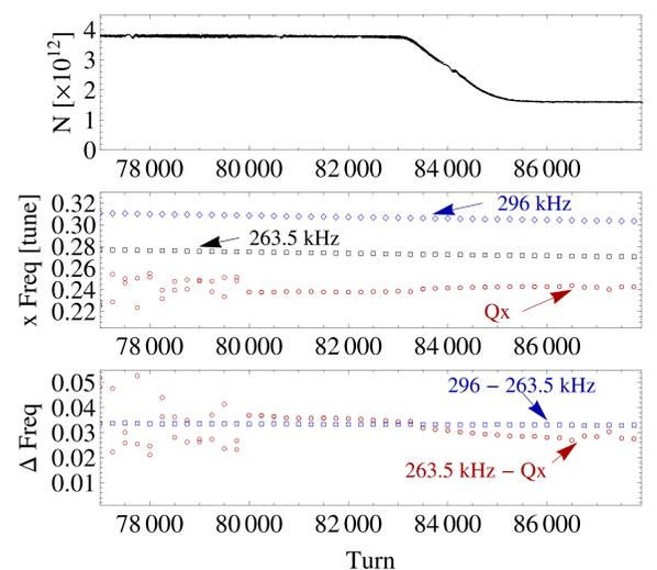
Top: Beam intensity near instability at  $c = 390$  ms. Center:  $Q_x$  and tunes of 263.5 and 296 kHz lines. Revolution frequency is increasing, so tunes of fixed-frequency lines are changing. Bottom: Difference between tune of 263.5 kHz line and  $Q_x$ , and between tunes of 296 and 263.5 kHz lines. Beam loss begins precisely when the differences between all three spectral lines are equal.
