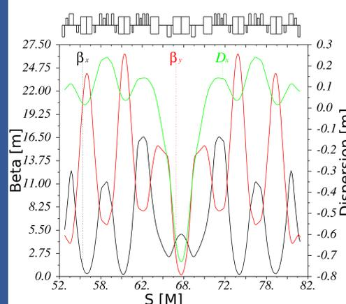
A chicane placed in one long straight section zero the  $\alpha$ :
