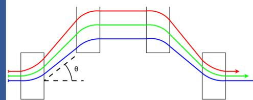
4 dipoles arranged in a chicane. Electrons with higher energy travel through longer paths than electrons with lower energy, resulting in a negative momentum compaction factor.
