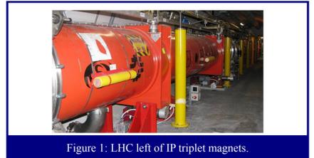
Figure 1: LHC left of IP triplet magnets.
