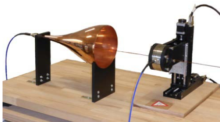
Current Transformer testing on the Goubau Line
