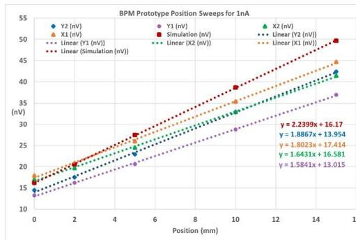
Position Sensitivity comparison between simulation and test bench for positive displacements.
