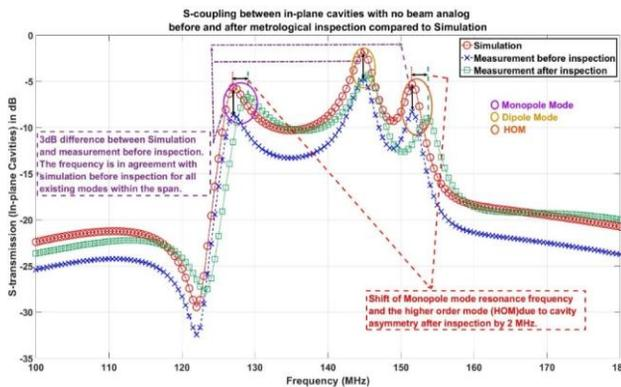
S-transmission between in-plane cavities in the absence of beam analog before and after mechanical reassembly compared to Simulation.
