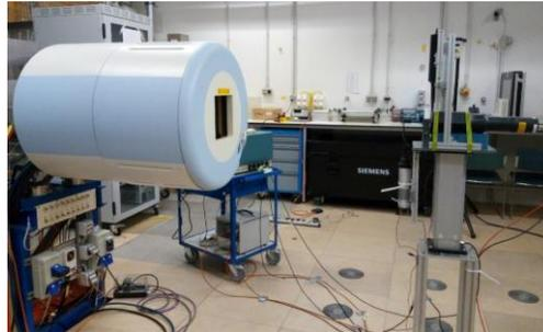
Experimental setup mounted at HIT (Germany), and used for mass- and charge-changing cross section measurements. The detection system was designed at GSI.
