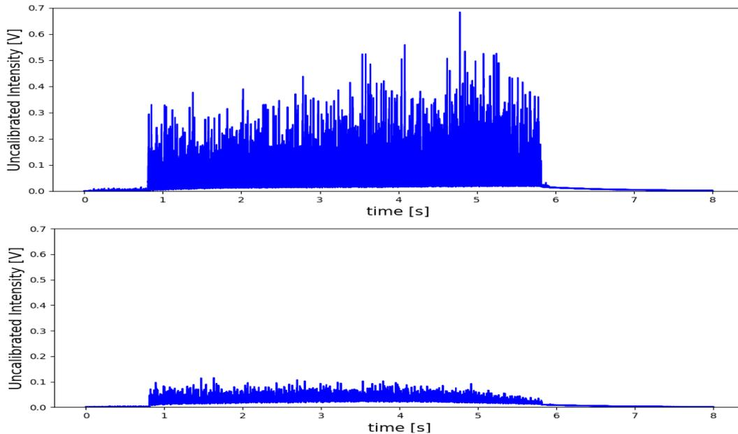
Extracted beam intensity over time, 50kHz sampling. (top) Reference (bottom) with RF-channelling. Same integrated intensity, or comparable with shot-to-shot variations.
