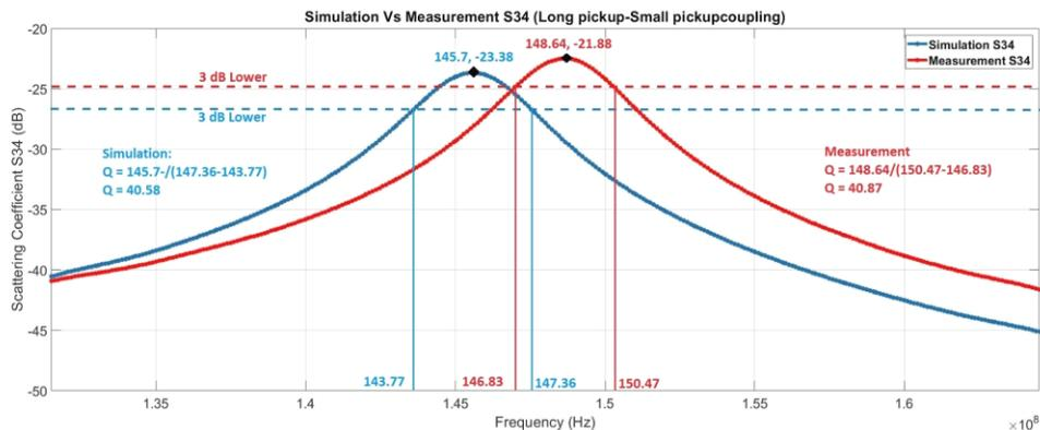
Comparison of Scattering parameter S34 between a long and a short pickup between simulation and measurement
