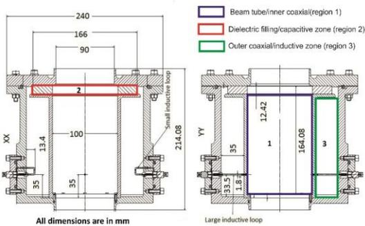
*Dielectric-filled reentrant cavity resonator with induced E and B fields in the separate capacitive and inductive zones*
