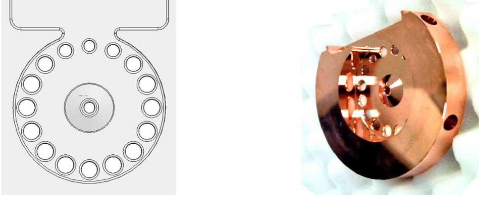
Figure 2.2: Input coupler design (left) and single mechanical cell (right) of the S-band BTW HT.
