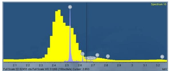
Figure 3: Synthesized material containing Bismuth and Chlorine – EDS spectrum (yellow), and WDS spectrum (purple)
