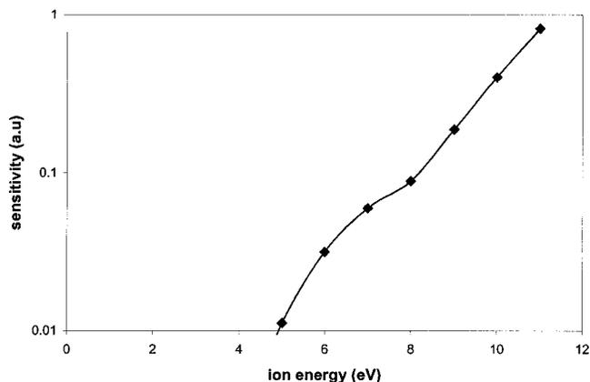
FIG. 6. Sensitivity (in arbitrary units) against ion source voltage for the same conditions and spectra as shown in Fig. 3.
