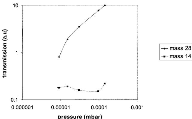
FIG. 9. Transmission (in arbitrary units) against pressure for nitrogen spectra in the pressure range to  $10^{-3}$  mbar and ion source emission current 0.5 mA.
