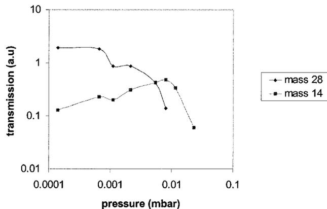
FIG. 10. Transmission (in arbitrary units) against pressure for nitrogen spectra in the pressure range to  $10^{-1}$  mbar and ion source emission current 0.2 mA.
