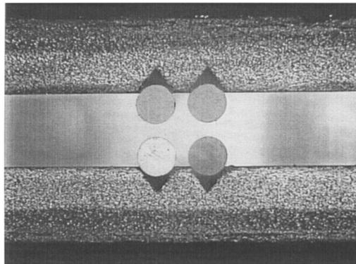
FIG. 1. End on view of the MEMS mass filter. The four QMS electrodes are 0.5 mm diameter, metal coated optical fibers bonded within etched V grooves in two silicon wafers.
