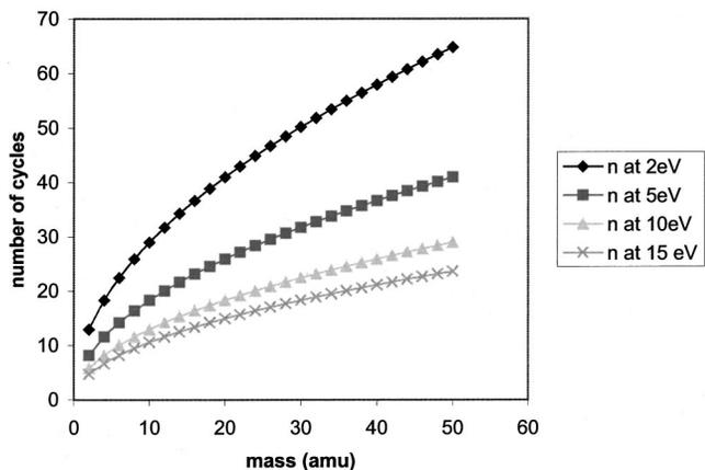
FIG. 8. Predicted number of rf cycles experienced by the ions in the MicroQuad mass filter of length 30 mm and rf 6 MHz as a function of  $m/e$  for different ion energies.
