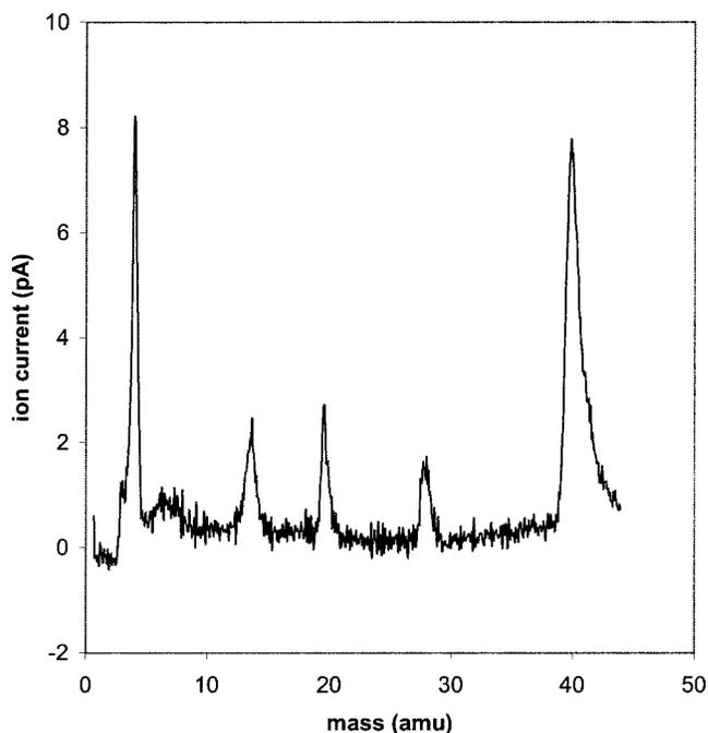
FIG. 3. Mass spectra obtained from the output of the electrometer for an argon/nitrogen/helium gas mixture. Total pressure  $2 \times 10^{-5}$  mbar, ion source voltage 13.5 V, emission current 2 mA, and pole bias 8.7 V.
