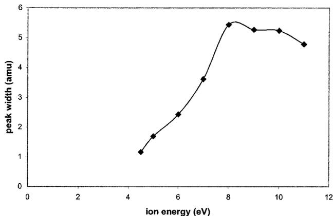
FIG. 5. Peak width at 10% peak height against ion source voltage (ion energy) for a range of argon spectra. Emission current 0.2 mA and pressure  $5 \times 10^{-5}$  mbar.
