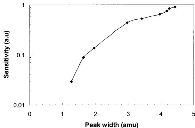
FIG. 7. Sensitivity (in arbitrary units) against peak width at 10% peak height for varying  $U/V$  voltage ratios for the same conditions and spectra as shown in Fig. 3. Ion source voltage 8.7 V, pole bias 7 V, ion source emission current 0.2 mA, and pressure  $3 \times 10^{-5}$  mbar.
