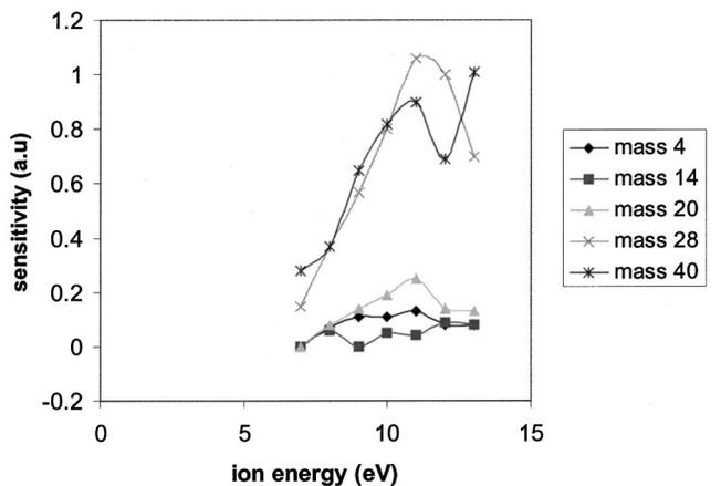
FIG. 4. Effect of ion energy on sensitivity (in arbitrary units) for constant source voltage and varying dc pole bias to the QMS rods.
