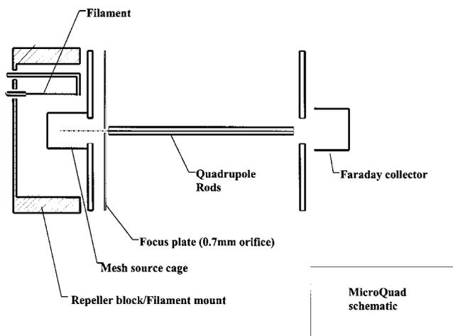
FIG. 2. Schematic diagram of the MEMS mass filter assembled in line with a conventional hot filament ion source and Faraday collector to form the MicroQuad.
