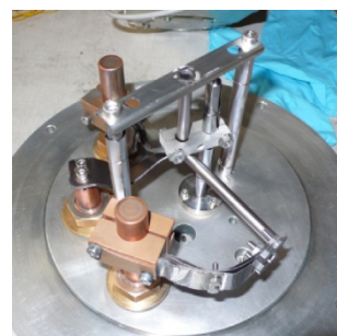
LISBET is the new RILIS off-line ion source at GANIL.
