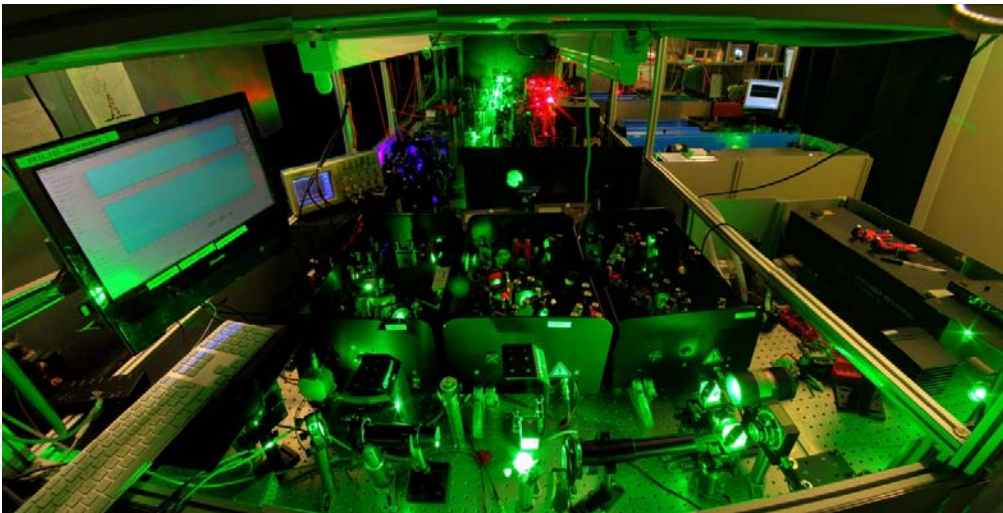
The photograph shows the Dual RILIS laser setup. Three Ti:Sa laser cavities (front) are simultaneously pumped by a frequency doubled Nd:YAG laser (right, front). Two of the three dye lasers as well as the dye pump laser were placed on extensions to the main laser table (right, top).
