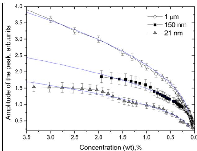
The experimental influence of the concentration of TiO<sub>2</sub> seeders in the flow of water on the spectrum of the self-mixing signal with a fixed flow velocity (at 1.3 m/s).
