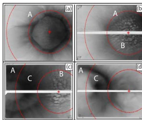
Proton spatial-intensity profiles in the energy range 5–7 MeV, in different conditions of the interaction.
