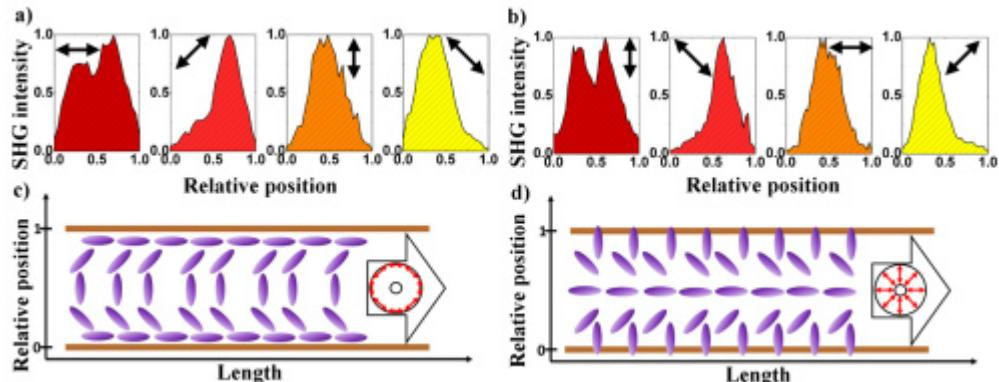
Normalized SHG intensities as a function of the normalized line thickness for (a) azimuthally polarized irradiation and (b) radially polarized irradiation. Cross-sectional scans for different excitation beam (1064 nm) polarization directions - indicated by black arrows. Simplified depiction of the Ag ellipsoids orientations (c) and (d) within the line cross section according to (a) and (b) for both irradiation polarization directions - shown with red arrows.
