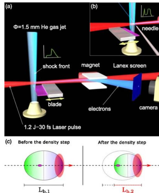
Schematic representation of the first (a) and second (b) experimental setup. The blade can move in and out the gas jet. The density profile is shown in green in the two cases near the gas jet. (c) Schematic representation of the bubble before and after the density step.
