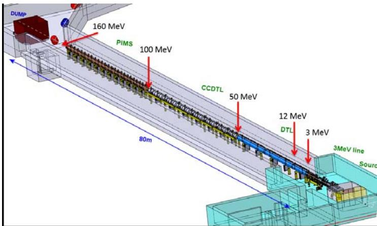
LINAC4 facility indicating the beam energy that will be reached during the different commissioning stages. The laser stripping system has already been tested at 3 MeV and 12 MeV periods and is presently setup for 50 MeV and 100 MeV before being permanently installed at 160 MeV.
