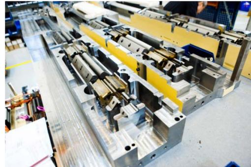
Compact magnet systems are smaller and thus the number of elements can be increased. This results in an extremely low emittance. The low emittance makes possible an extremely bright synchrotron light.
