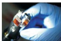
Photograph of an electro-optic GaP crystal, mounted on its support.
