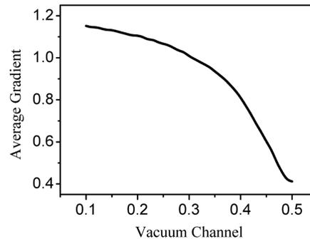
Optimum vacuum channel width; For this simulation, wall thickness and pillar height are chosen 0.5 and 0.9 laser wavelength, respectively
