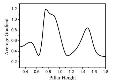
Optimum pillar height; For this simulation, wall thickness and vacuum channel width are chosen 0.5 and 0.24 laser wavelength, respectively
