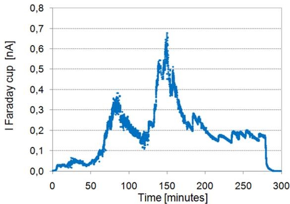
FIG. 5. Ion current detected for  $^{64}\text{Zn}$  during the efficiency measurement.
