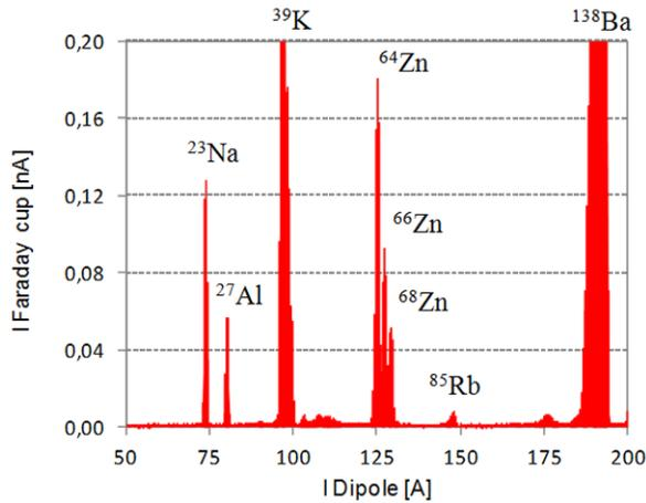
FIG. 4. The complete mass spectrum of ions coming out the ion source. All peaks except zinc are produced by the surface ionization.
