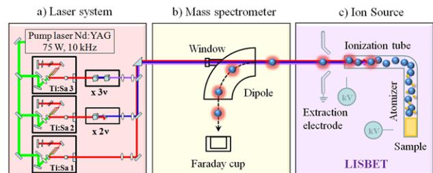
FIG. 1. (Color online). General setup for GISELE test bench: a) laser system, b) mass spectrometer c) LISBET ion source.
