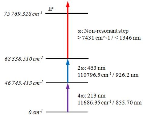
FIG. 3. (Color online) Ionization scheme for zinc atoms with a non-resonant third step transition.
