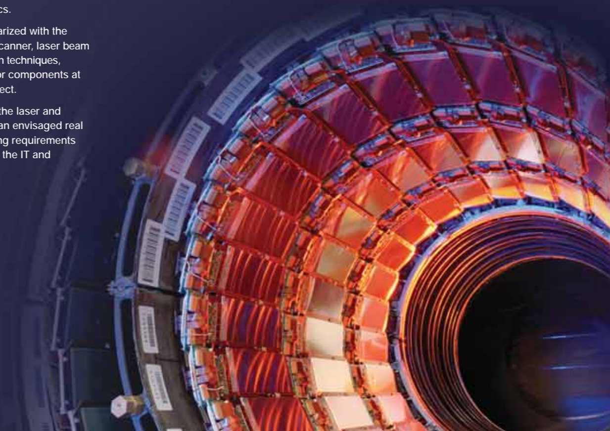
First half of CMS inner tracker barrel at the LHC © 2006 CERN
